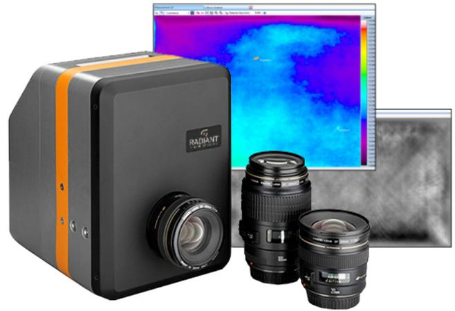
*The ProMetric® I Imaging Colorimeter captures complete 2D images of a part under test, applying a sequence of measurements in TrueTest™ Software for comprehensive evaluation in seconds.*
