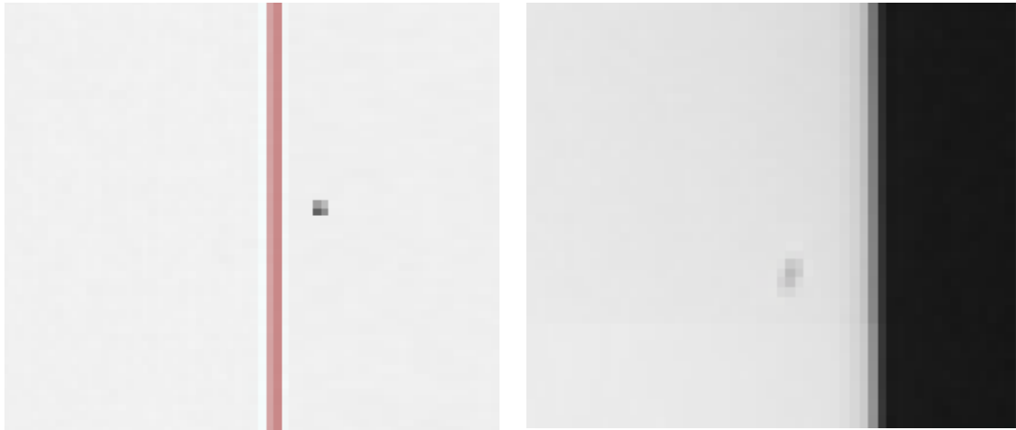
Pixel defects captured in an image of a 1500R curved display from 0,0 perpendicular position (poor resolution/DOF applied)
