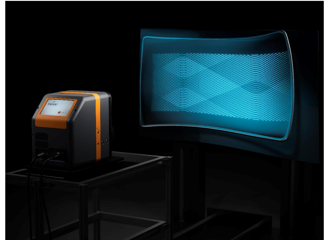
Example measurement setup; ProMetric I Imaging Colorimeter measuring curved glass from 0,0 perpendicular position.
