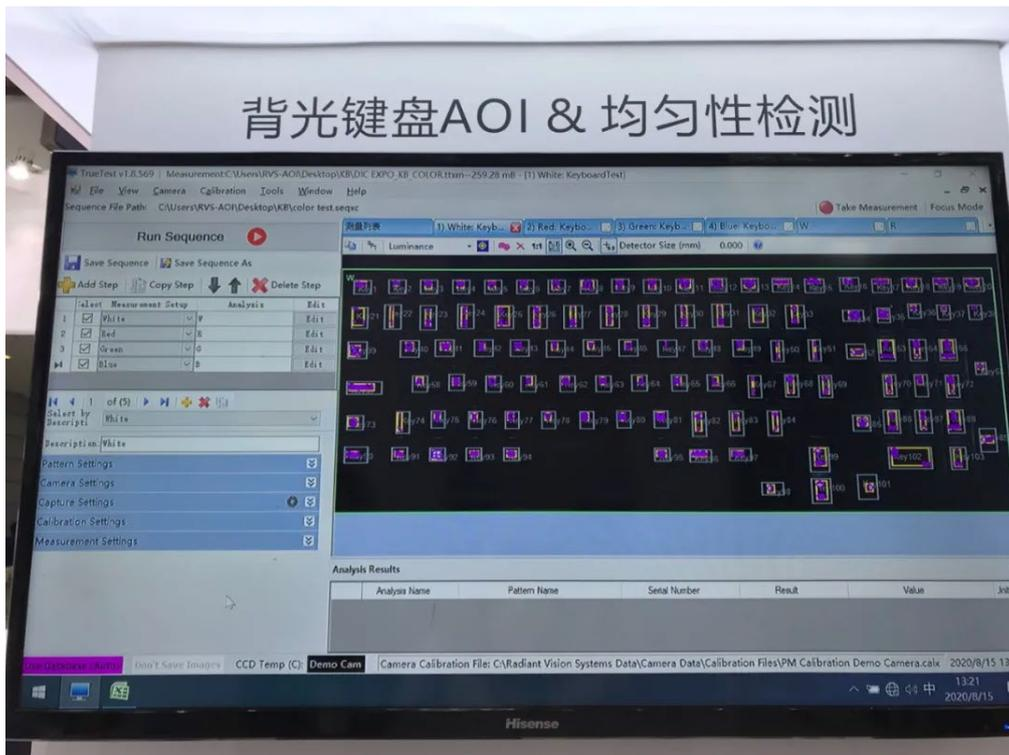
*Radiant's keyboard inspection software demonstrated from the floor of CITE 2020. All keys and characters are measured simultaneously for brightness, color, and dimensional quality.*
