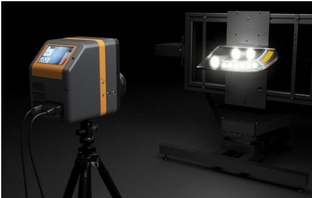
Figure 4 – Measuring luminous flux at all angles of an automotive headlamp using a ProMetric imaging colorimeter and a goniometer for near-field data in a small dark room.
