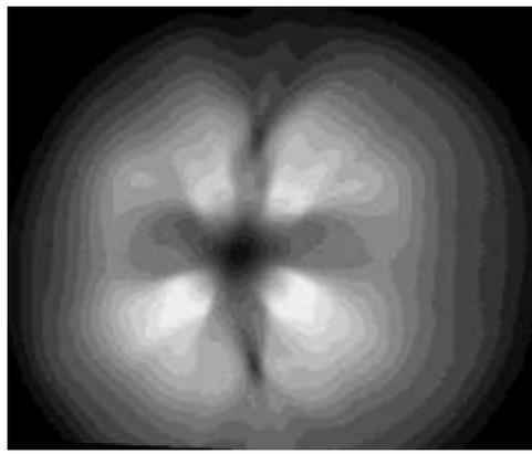
**Figure 5 Actual measurement of HPL lamp in ellipsoidal reflector**
