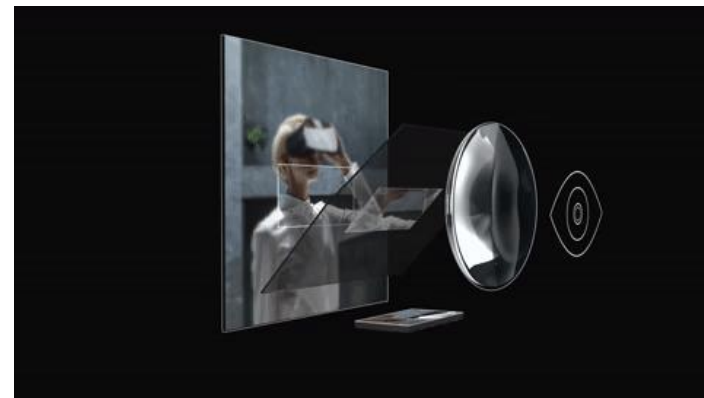
Example of foveated optics from Varjo using two displays and a rotating combiner to adjust focal point. (Source: RoadtoVR )
