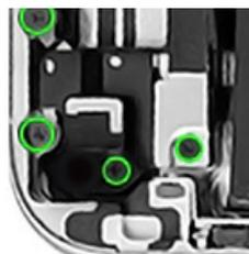
**Escaped:** The traditional machine vision camera does not distinguish a black hole from a black screw, and the defective assembly escapes.
