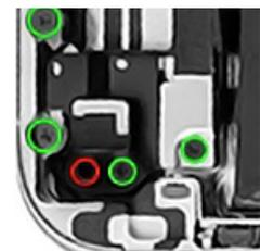
**Detected:** The photometry-based imaging system detects the missing screw, and the defective assembly can be corrected or rejected before progressing.
